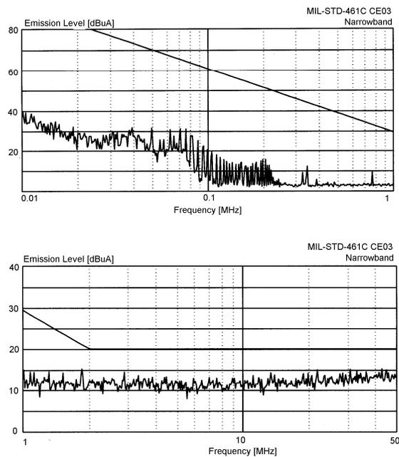
**Figure 10 – DVWR2800T with EMI Filter**
