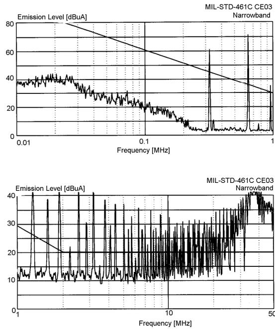
**Figure 9 – DVWR2800T without EMI Filter**
