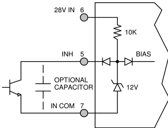
**Figure 4** – Internal Inhibit Circuit and Recommended Drive
