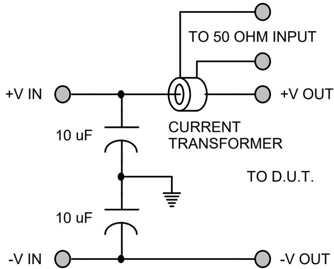
Figure 5 – MIL-STD-461C Measurement Method (Feedthrough Capacitor)
