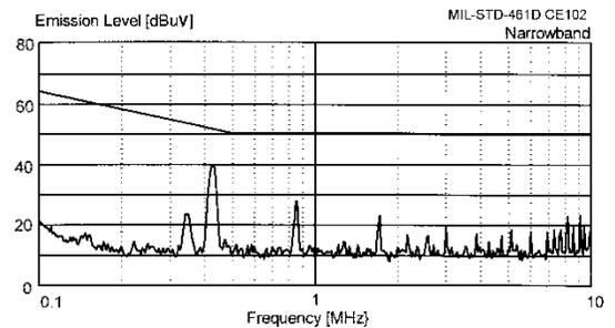
**Figure 10 – MIL-STD-461D DVHF2800S With DVMH28 EMI Filter**
