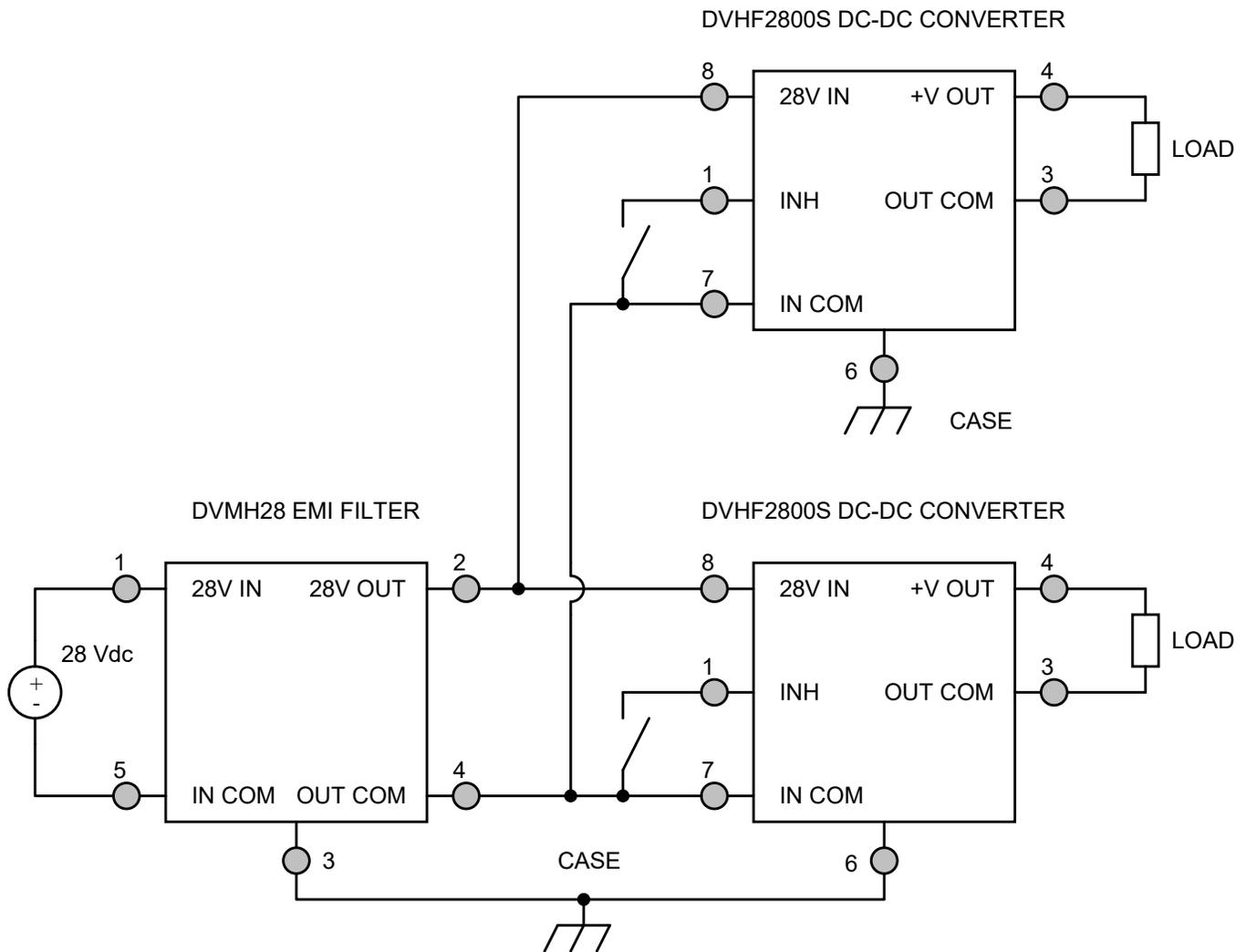
Figure 4 – DVMH28 EMI Filter Hookup with Two Converters
