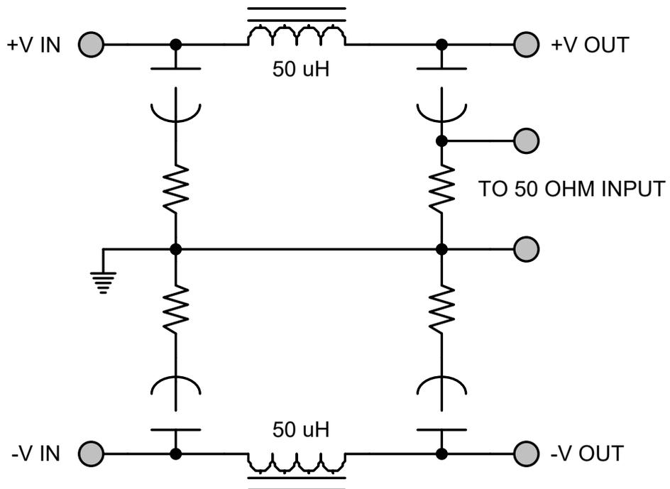
Figure 6 – MIL-STD-461D Measurement Method (LISN)
