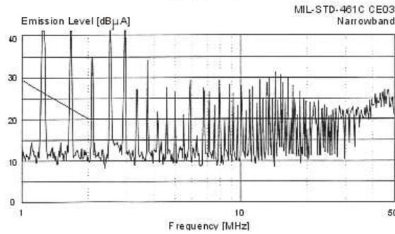
**Figure 7 – MIL-STD-461C DVHF2800D Without EMI Filter**
