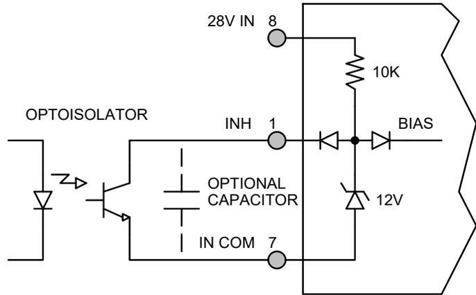
**Figure 5** – Isolated Inhibit Drive
